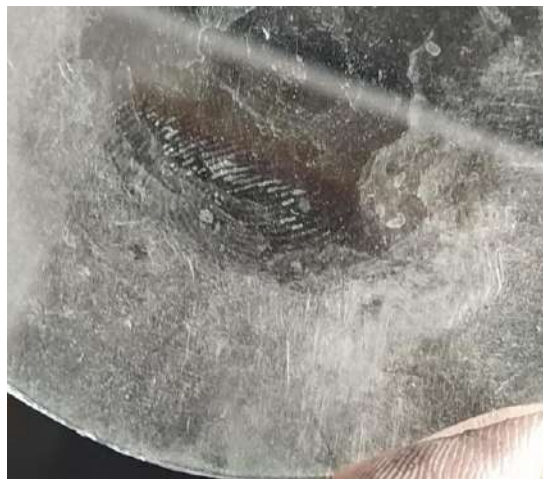
Figure 4: Petri-dish dipped in water for 1 hour and then developed with white powder
