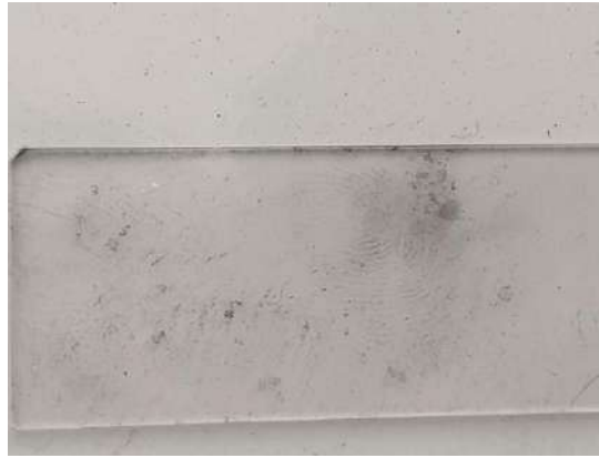
Figure 11: Glass slide dipped in dilute HCl for 2 hour and then developed with black powder
