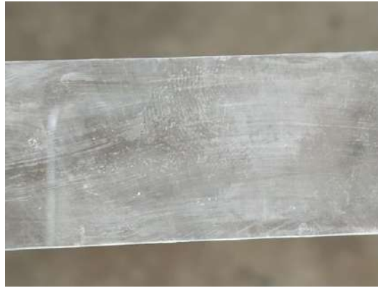
Figure 9: Glass slide dipped in dilute NaCl for 3 hour and then developed with white powder
