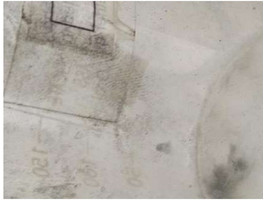
Figure 3: Beaker dipped in water for 3 hour and then developed with black powder
