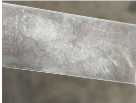
Figure 7: Glass slide dipped in dilute NaCl for 1 hour and then developed with white powder
