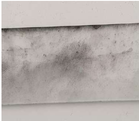
Figure 10: Glass slide dipped in dilute HCl for 1 hour and then developed with black powder
