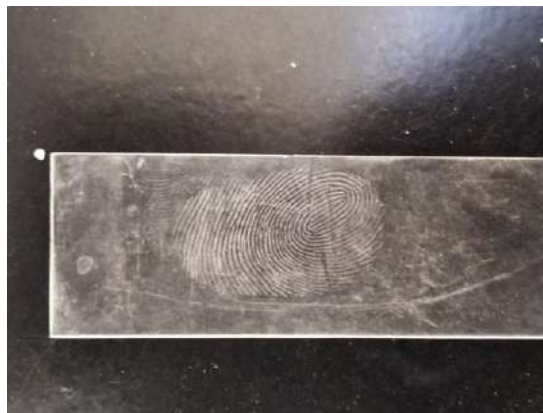
Figure 8: Glass slide dipped in dilute NaCl for 2 hour and then developed with white powder
