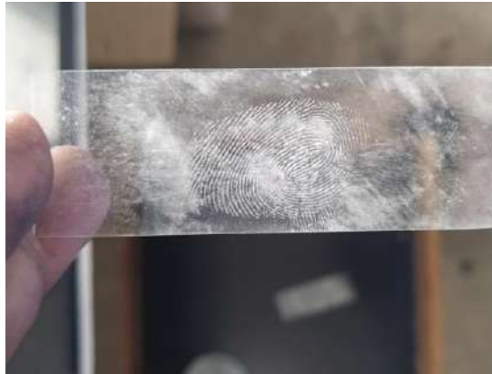
Figure 5: Glass slide dipped in water for 2 hour and then developed with white powder
