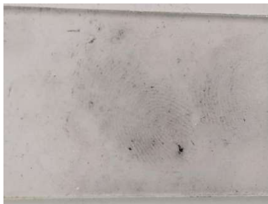
Figure 12: Glass slide dipped in dilute HCl for 3 hour and then developed with black powder
